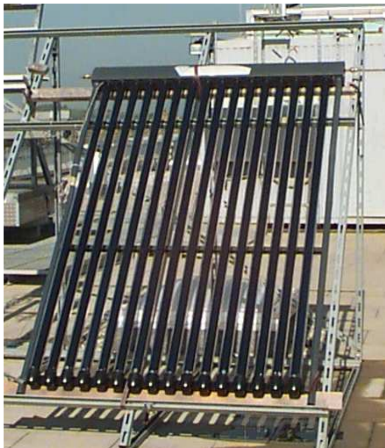
Figure 1: Picture of the collector HJJ 16/2.1 mounted on the test facility of Fraunhofer ISE
